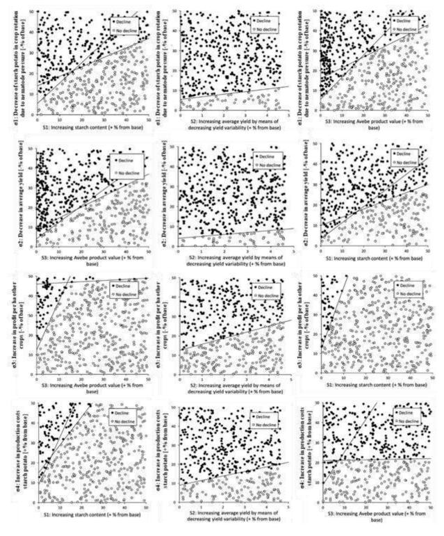
Figure 4.22: Simulation results of strategies (S1, S3) in combination with different disturbances. A threshold line shows the minimum relative change of a strategy parameters that is required to prevent a system decline given a relative change of a challenge parameter. A system decline occurs when starch potato production decreases by more than 20% from the 2020 value in 2050.
